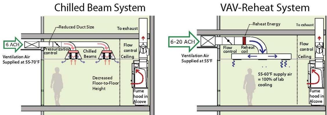
Figure 34: Chilled Beam vs. VAV-Reheat systems in laboratories. From Labs21: Chilled Beams in Laboratories
