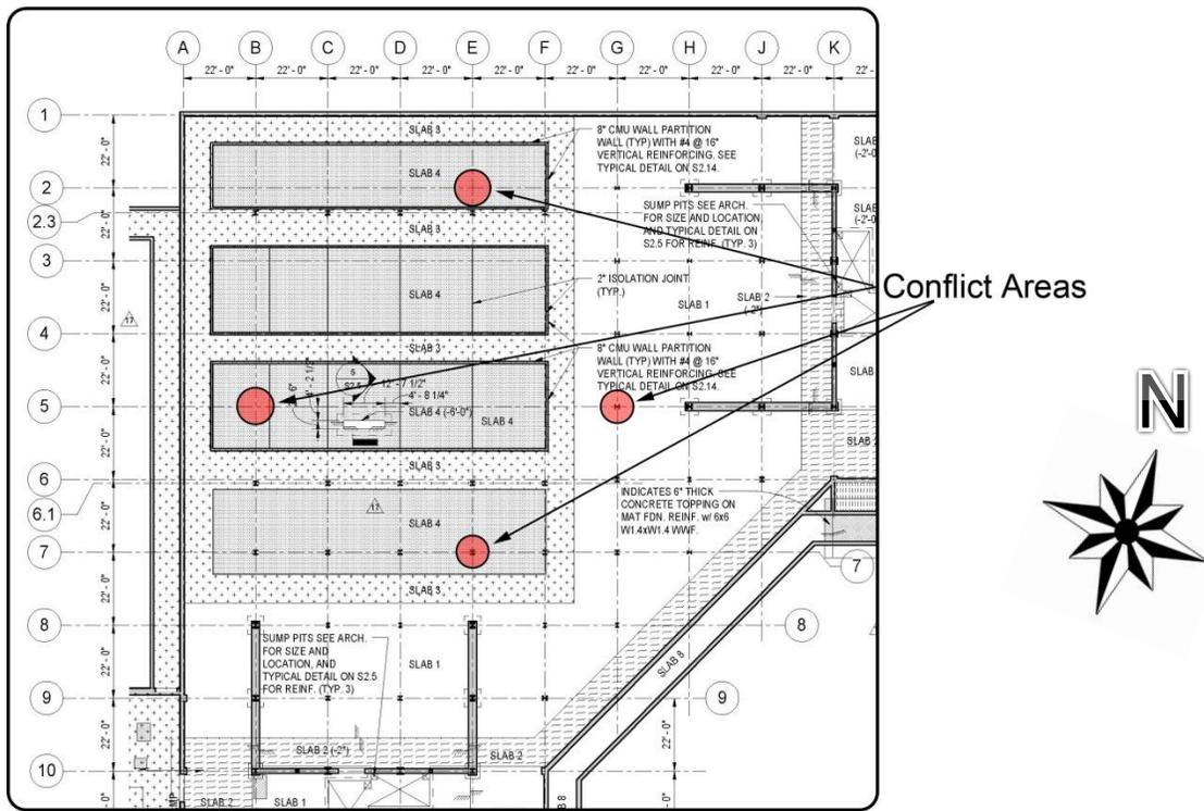
**Figure 43: Locations where cantilever bracing will meet the basement floor and the pile caps: Isolation slabs, beams and existing column conflicts resolved through minor offsets**
