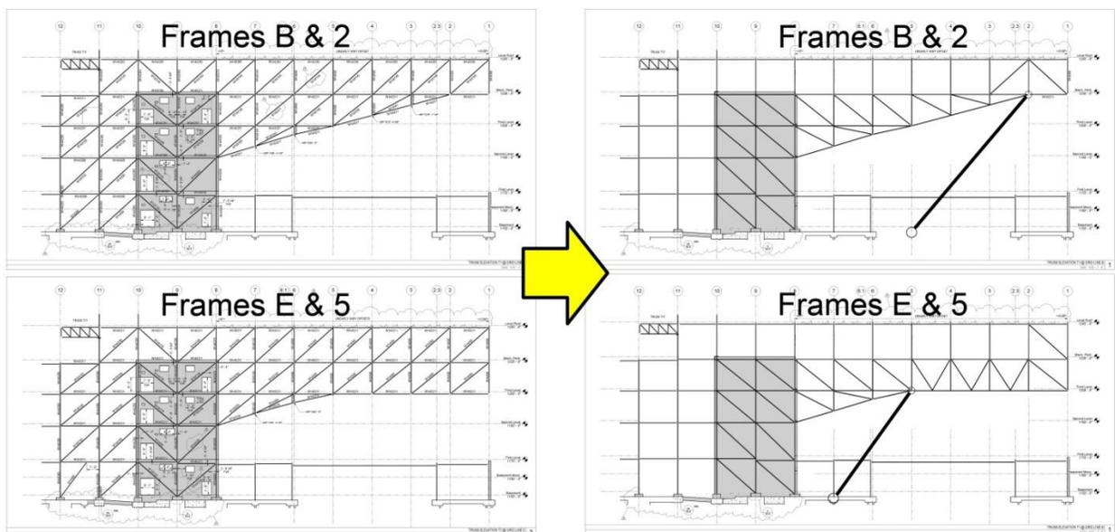
**Figure 42: Columns would be placed at each truss frame, eliminating the need for many of the braces in the current configuration**
