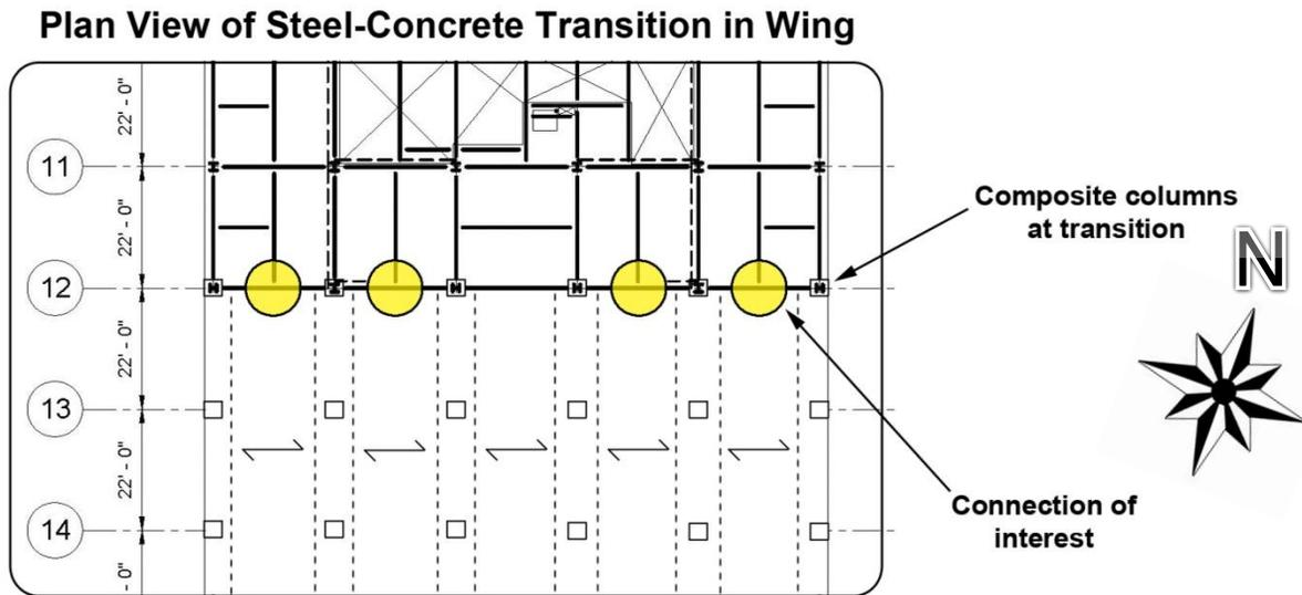
Figure 40: Transition at grid line 12
