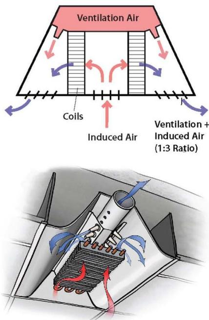
**Figure 33: Proposed Active Chilled Beam. From Labs21: Chilled Beams in Laboratories**
