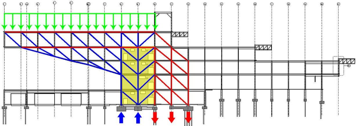
Figure 20: Special Systems load distribution
