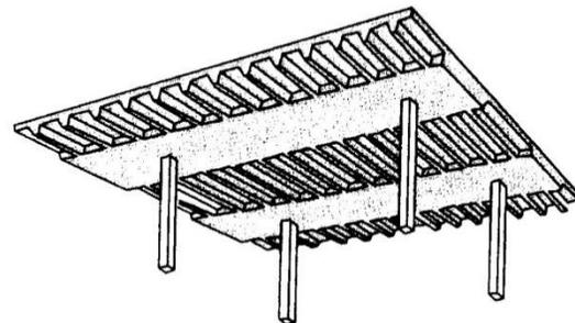
Figure 37: Pan Joists
